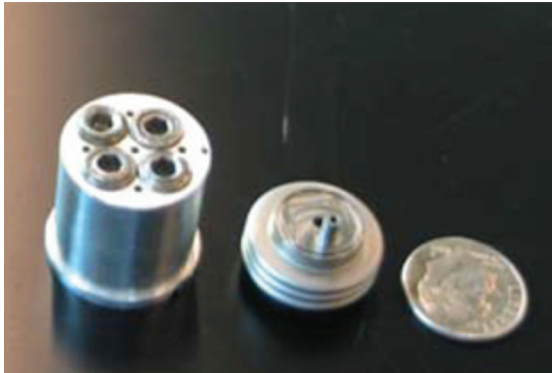
Images: Melt cell technology. Melt cells contain materials that provide temperature calibration by nature of their precise phase change characteristics. Left image: Two space flight cells (next to dime, for size reference). The melt cells will be placed in a special container (right image) before being sent to the International Space Station.
